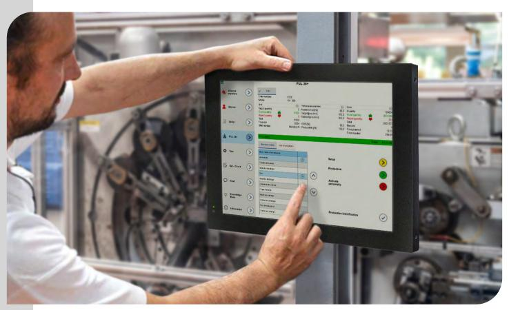
The MES terminals on the shopfloor make it easier for workers to work. They provide information about current and planned orders and are easy to operate thanks to a self-explanatory user interface with touch screen function. Workers are relieved of handwriting and have a record of their work.
