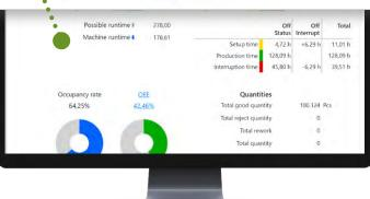
**Exact machine running times and setup, production and interruption times supplement the all-round view.** Weak points can thus be quickly identified and enable the targeted use of optimization measures.
