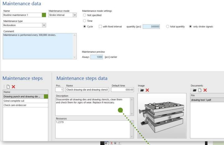
Maintenance cycles can be set up and defined in EMC.Maintenance according to precise criteria such as production quantity, cycles or operating hours. If maintenance is imminent, it is automatically reported via the MES Software EMC and a maintenance order is generated.
